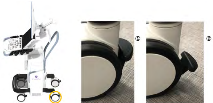
Figure 3-43. Left-rear caster
